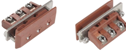
Type K illustrated (F35K). Recommended cutout: 8.5mm x 24.3mm
