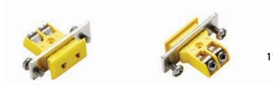
Type K ANSI illustrated (M29K-A). Recommended cutout: 6mm x 14mm
