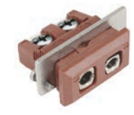
Recommended cutout: 13mm x 26mm. Type K illustrated (R34K)
