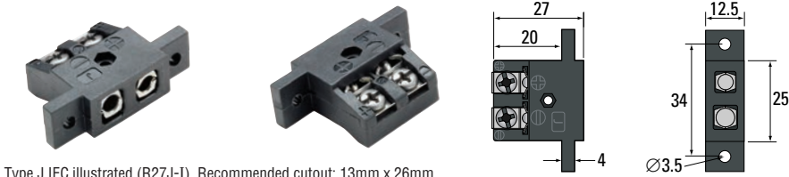
Type J IEC illustrated (R27J-I). Recommended cutout: 13mm x 26mm
