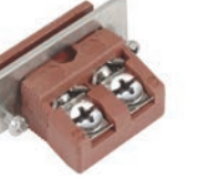
Recommended cutout: 13mm x 26mm. Type K illustrated (R34K)
