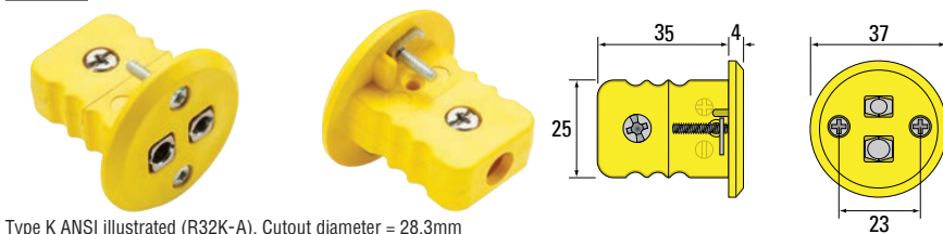
Type K ANSI illustrated (R32K-A). Cutout diameter = 28.3mm
