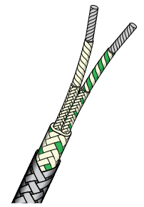
High Temperature Fibreglass Flat Twin with Stainless Steel Braid One pair of stranded conductors. Cores double HT glass fibre lapped, braided and varnished. Pair laid flat, HT glass fibre braided & varnished. Stainless steel wire braided overall.
