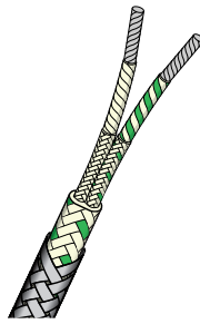
Fibreglass Flat Twin with Stainless Steel Braid One pair of stranded conductors. Cores double glass fibre lapped, braided and varnished. Pair laid flat, glass fibre braided and varnished. Stainless steel wire braided overall.
