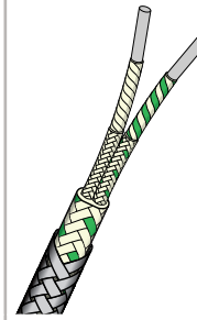
High Temp. Fibreglass Flat Twin with Stainless Steel Braid One pair of solid conductors. Cores single HT glass fibre lapped, braided and varnished. Pair laid flat, glass fibre braided and varnished. Stainless steel wire braided overall.
