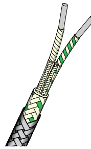
High Temperature Fibreglass Flat Twin with Stainless Steel Braid One pair of solid conductors. Cores double HT glass fibre lapped, braided and varnished. Pair laid flat, HT glass fibre braided & varnished. Stainless steel wire braided overall.
